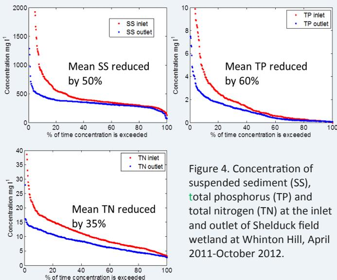
Figure 4. Concentration of suspended sediment (SS), total phosphorus (TP) and total nitrogen (TN) at the inlet and outlet of Shelduck field wetland at Whinton Hill, April 2011-October 2012.
