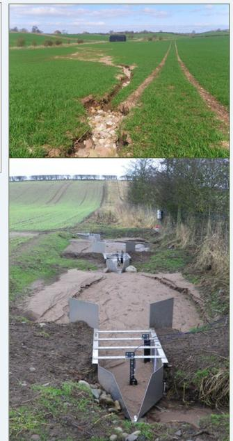
Figure 3. Gully erosion in 2010 (top right) resulted in the complete filling of Gully Trap wetland (bottom right) which was later dredged out.
